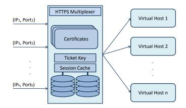
Fig. 1. Design of an HTTPS multiplexer
